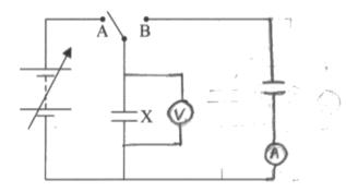
When the switch is connected to terminal A the capacitor X is connected to the variable power supply.
