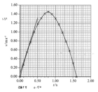
(b) (i) Draw a tangent to the graph at t = 0.40 s and use it to calculate the acceleration at this point.
